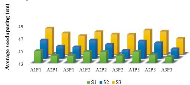
Fig. 3 : Effect of inclination angle, geometry of seed hole and forward speed on the average spacing of cotton seed.
