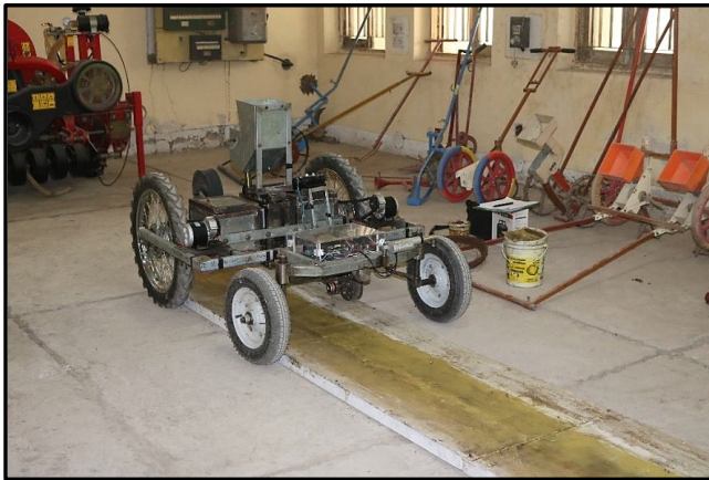
Fig. 2 : Experimental setup for laboratory evaluation of developed planter.
